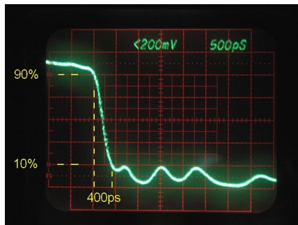
Fig. 12: Positive output fall time
