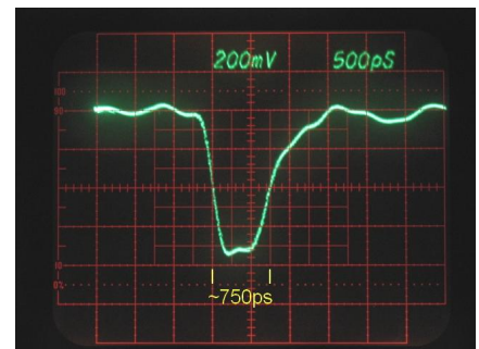
Fig. 9: Shaped neg. out min. width
