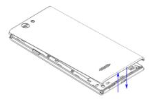
Hold the SIM card with the cut corner oriented as shown, and slip it into the card holder.
