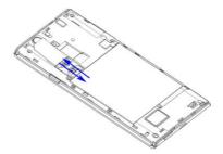
3. Insert the memory card into the metal slot with the metal contacts facing down until it clicks to the right position.
