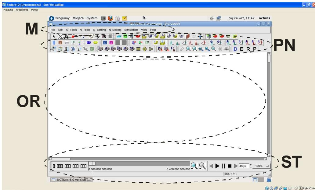
Fig. 4 Main elements of NCTUns program GUI
