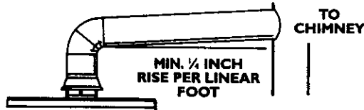
VENT PIPE INSTALLATION
