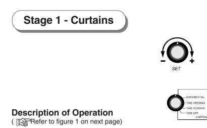
When the room temperature rises to "temperature set point + differential" (point 1), the curtains begin to open and continue to do so as long as the room temperature remains above this point. The curtains open intermittently according to the time opening and time off settings:
