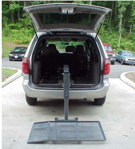
Platform resting properly on level ground
