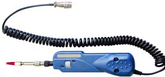
FVO-600A video microscope is used to inspect end-face of fibers and check the optic connectivity. It magnifies fibers of 125um diameter 650 times, enlarging picture through a video signal to the display where the status of fiber end-face is showed clearly in the end.
