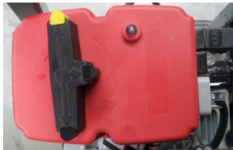
Figure 14 – Normally closed position
