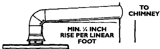
VENT PIPE INSTALLATION
