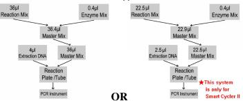
1) The volumes of Reaction Mix and Enzyme Mix per reaction multiply with the number of samples, which includes the number of the controls, standards and sample prepared. Molecular Grade Water is used as the negative control. For reasons of unprecise pipetting, always add an extra virtual sample. Mix the master mix completely then spin down briefly in a centrifuge. 2) Pipet **36µl (22.5µl for SmartCycer II)** Master Mix with micropipets of sterile filter tips to each
