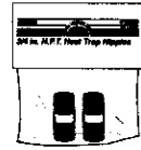
WATER HEATER HEAT TRAPS HELP REDUCE HEAT LOSS DUE TO THERMAL SYPHONING
