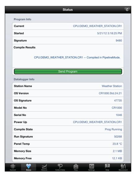
Note that a red E on the Status icon indicates that the datalogger has errors. Scroll down on the Status screen to identify the error.
