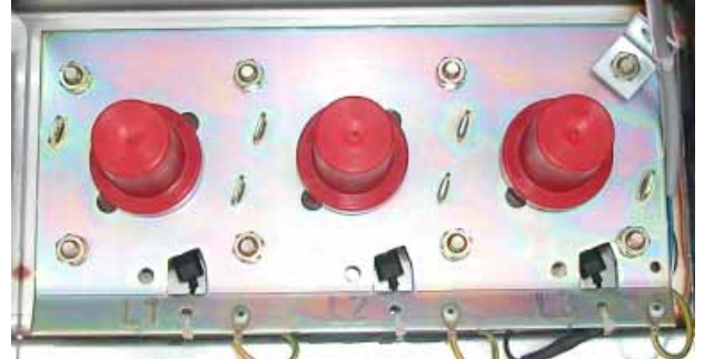
T1 (basic): Plug-in cross member PF250 NF-EN 50181, Connector - Type A (I r : 250 A, contact finger Ø M7.9 +0.02 / -0.05 mm)
