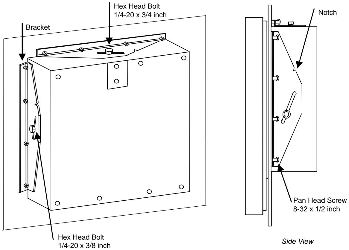
NOTE: Mounting brackets and attaching hardware are included in kit 30755065-502; panel gasket supplied in kit 51197657-501.
