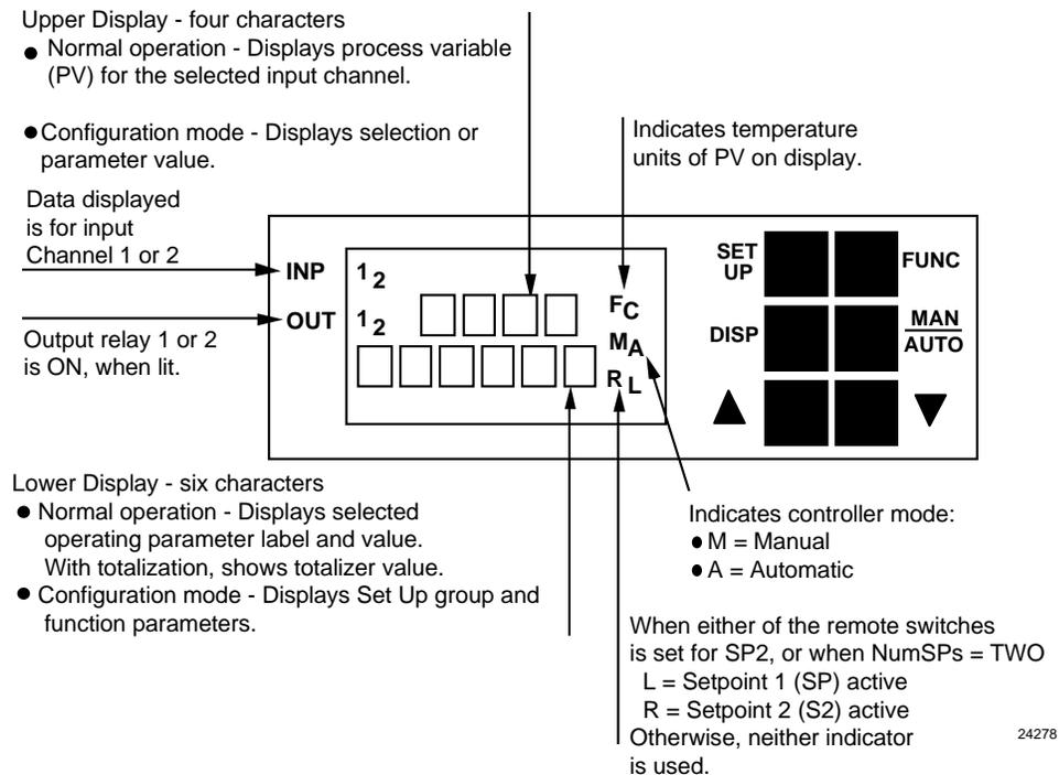
Figure 4-7 Operator Interface
