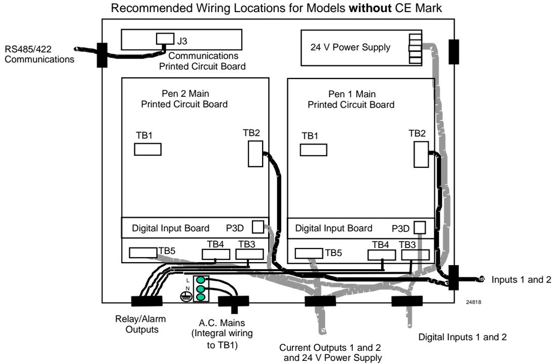
**Figure 2-7 Recommended Wiring Routing - Models Without CE Mark**
