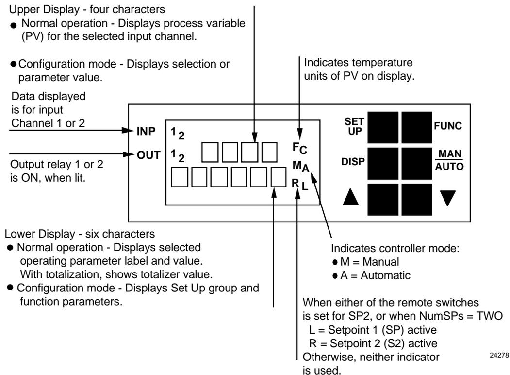
Figure 4-1 Operator Interface
