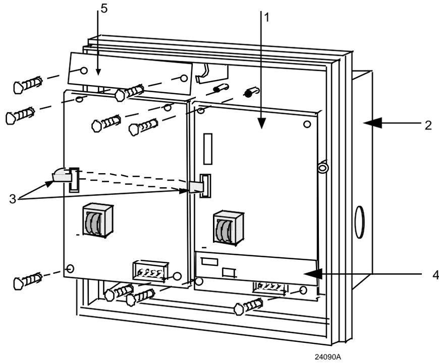
**Figure 9-3 Recorder Components**
