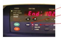
During a run the **RUN TIME** can display either the elapsed time, **E** or the remaining time, **R**.
