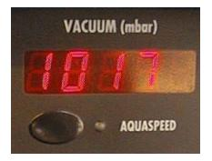
The vacuum display indicates the absolute pressure of the system in millibar (mbar).
