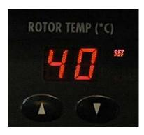
The maximum rotor temperature is monitored and controlled by the RotoGuard infrared temperature detection system.
