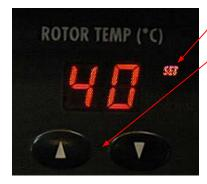
To change the setting, press both keys simultaneously and the SET prompt will flash.
