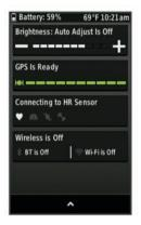
The connections page appears. A flashing icon means the device is searching. You can select any icon to change the settings.
