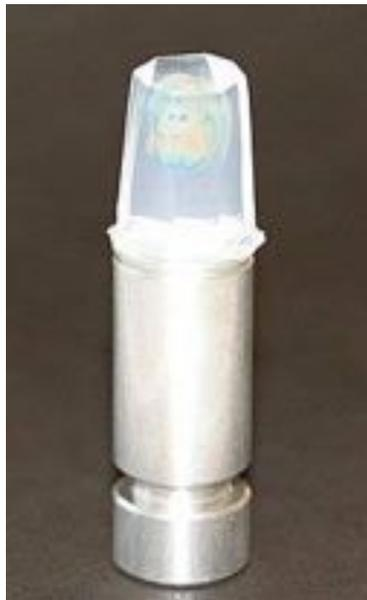
**Fig. A1j Trimmed Agarose Block on Mount**
