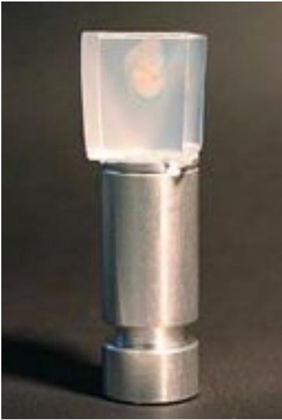
**Fig. A1f Agarose Block Attached to Mount**
