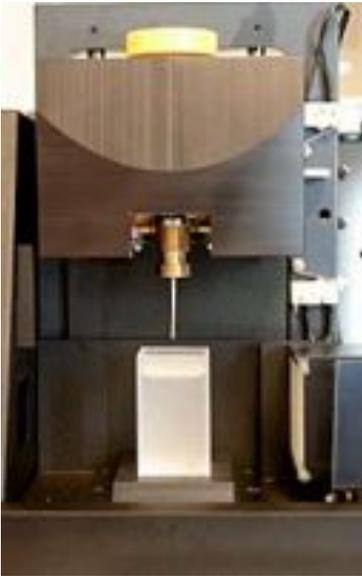
**Fig. 6a Alignment Pin attached to rotation stage**
