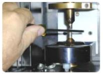
The electrode gap is the distance between the upper and lower. The gap should be no more than the width of a 5/32 Allen wrench. A 5/32 Allen wrench is the same tool used to loosen the screw that holds the upper electrode and is included with the analyzer's supplies.
