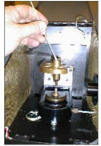
Use a cotton swap dipped in cleaning solution to clean the upper electrodes. First, wipe the outside of the upper electrode. Then, clean the inside of the upper electrode by inserting the swab down through the center of the electrode.
