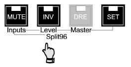
Once in *SET Inputs* mode (see above), press the *INV/Split96* button, to change the mode of inputs 2 and 3 for either Split96 (2-wire) or normal (1-wire) operation. In Split96 mode, two AES3 bearers both at 44.1kHz or 48kHz carry a stereo 88.2kHz- or 96kHz-sampled signal, with one channel carried on each bearer as described in ref. 8. "Split96" or "2-wire AES" sources may only be connected to Inputs 2 & 3.
