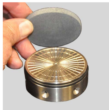
#170-69 Cell Cap, 2,000 psi, HTHP Filter Press Scribed For Ceramic Filters. Note: Round Set Screw Holes
