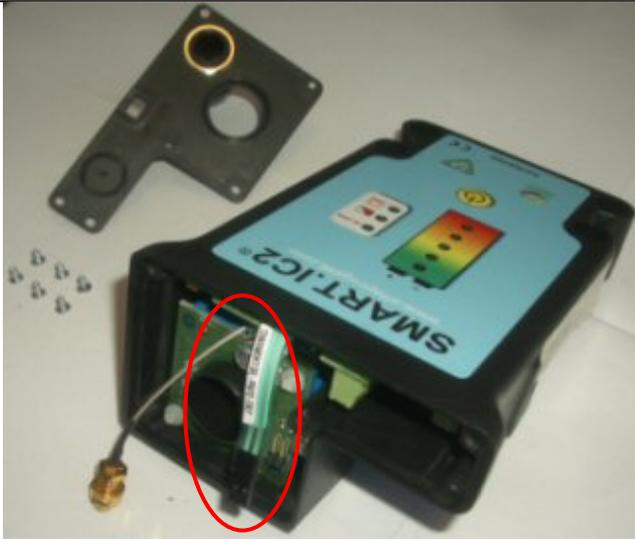
Disconnect the flat cable connector from the current sensor card.
