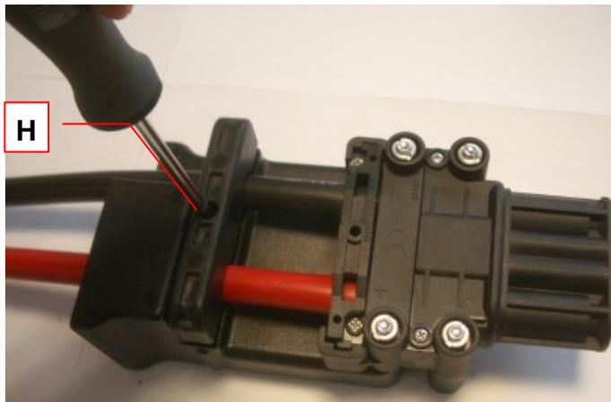
Close the clamp with the special cover (C), and secure it with the screw (H) supplied 3.5x16 mm (code V4).
