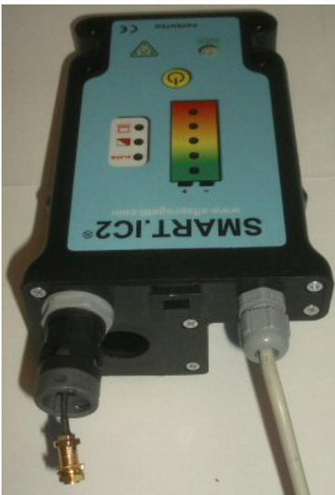
Reposition the electronic board in the container; connect the flat cable to the current sensor card. Close the back cover by tightening the 6 screws previously removed (code **V1**). Tighten the cable gland.
