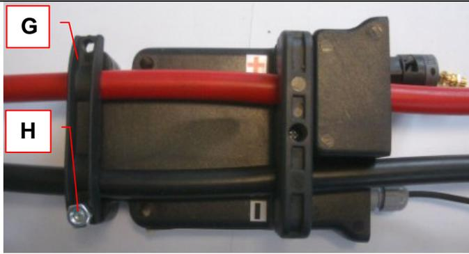
Also fasten the battery cables to the module (C) through the clamp collar (G) using screws (H) and fastening nuts (I).
