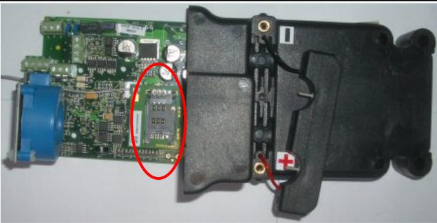
Remove the electronic board from the container until the slot for the SIM card is accessible.
