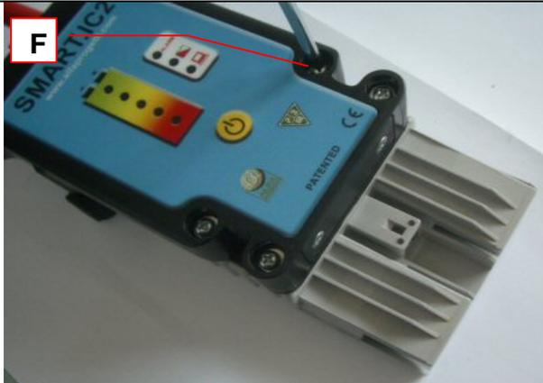
Fasten the adapter block **(D)** (code **P882EU**) to the SMART.IC2 with the 4 screws **(F)** and washers.
