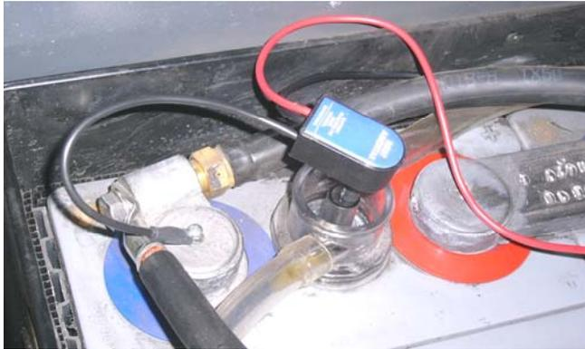
Place the level sensor within a cell of the battery (in the figure the automatic refilling cap was used; alternatively a hole can be made on the cell cap).
