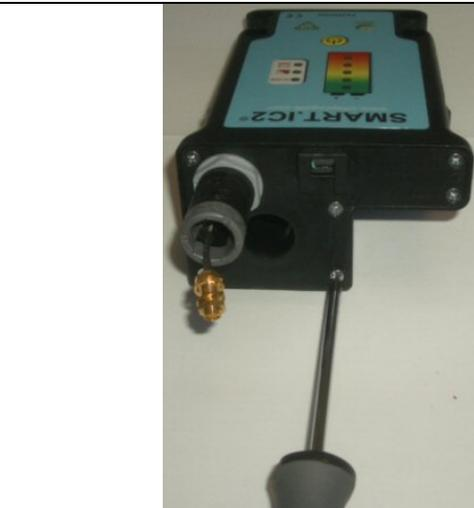
Replace the electronic board in the container; connect the flat cable to the current sensor card. Close the back cover and tighten the 6 screws previously removed (code **V1**).
