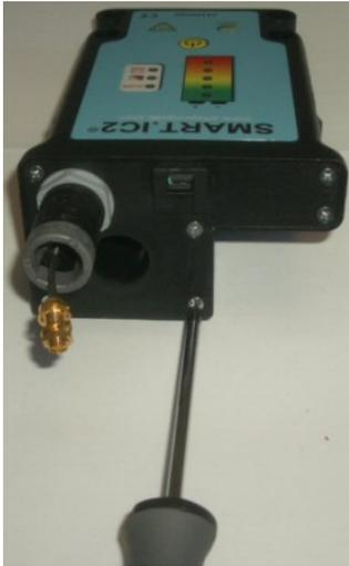
Remove the back cover by unscrewing the 6 screws (code **V1**).
