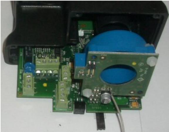
Remove the electronic board from the container until the green terminals next to the Hall sensor are accessible.
