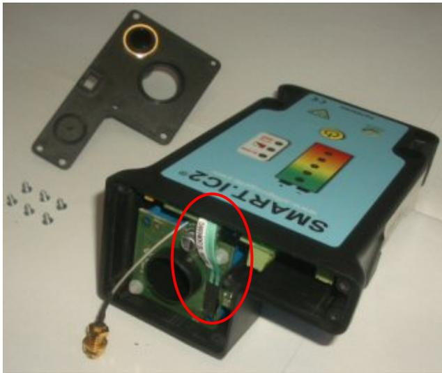
Locate the connector with a flat cable.
