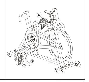
Assembly Step D Install the seat post (#9) into the frame receptor and secure with the knob
