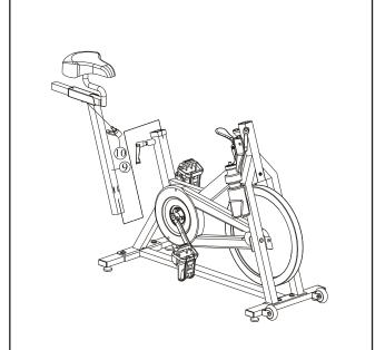
Assembly Step E Install the handlebar (#10) into the frame receptor and secure with the knob
