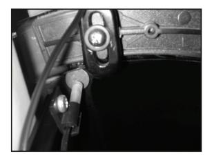
Insert the computer sensor wire into the RPM bracket then causes the wire to be away from the magnet on the flywheel 3 mm distance.
