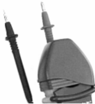
Fig. 3: Use of rubber test lead holster
