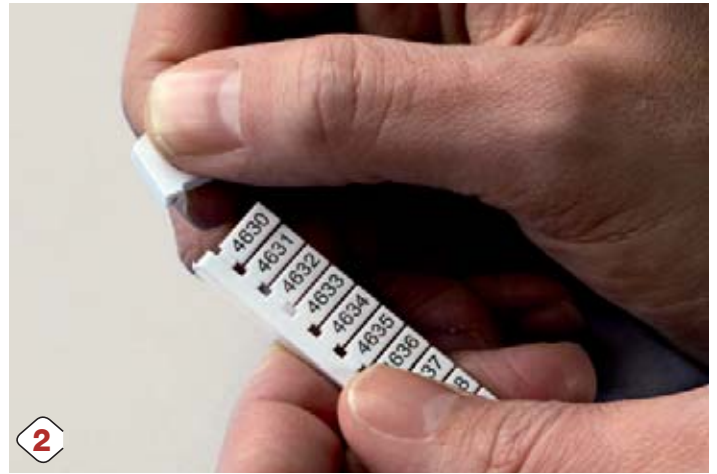
2 Remove the pre-notched heads from the stem.
