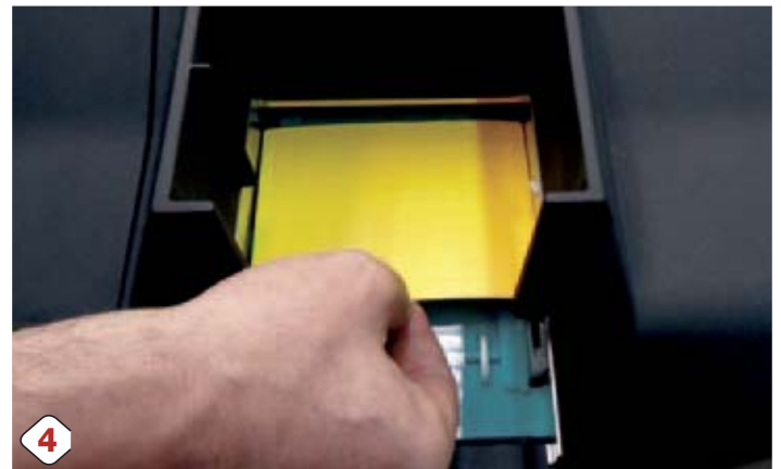
4 Place the labels directly onto the printing surface.
