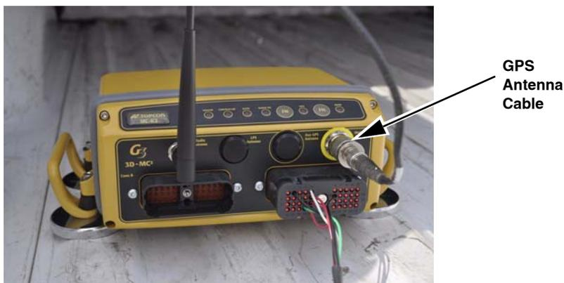
Figure 2-24. GPS Antenna Cable to MC-R3 Controller
