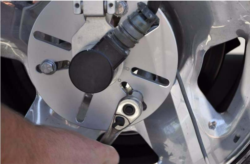
**Figure 2-7. Wheel Encoder Bolts**
