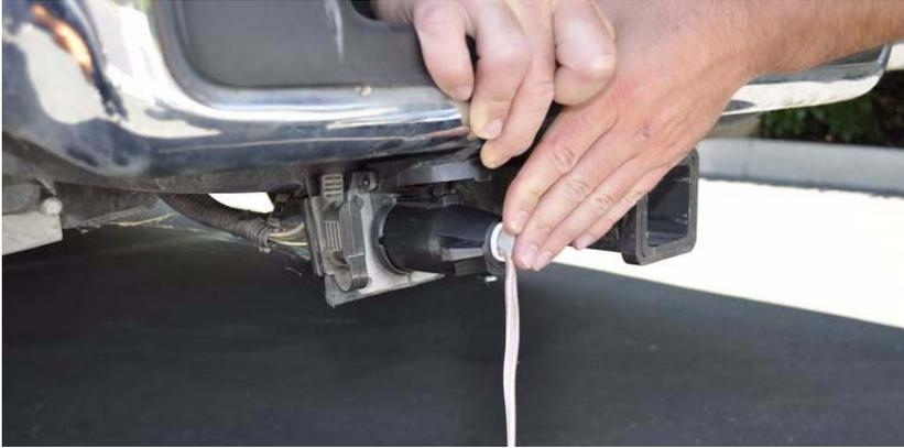
**Figure 2-17. RTP-300 Power Cable to Hitch**
