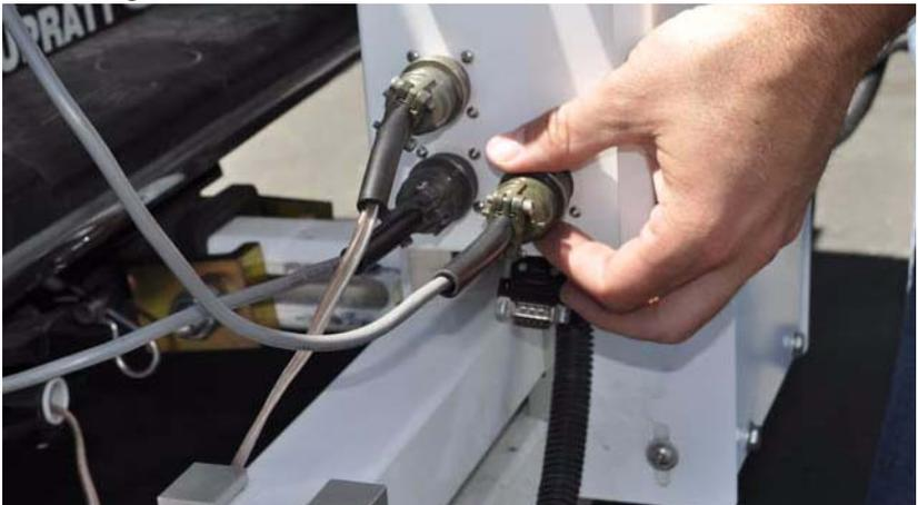
Figure 2-20. Communication Cable to RTP-300 Assembly
