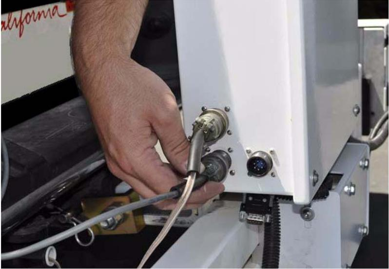
Figure 2-19. Wheel Encoder Cable to RTP-300 Assembly
