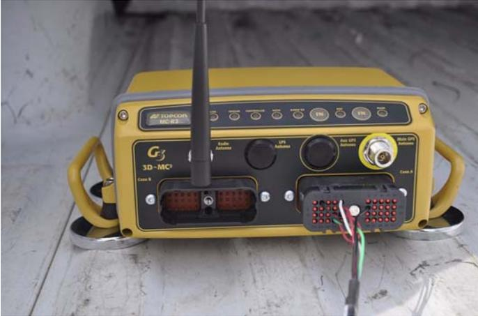
Figure 2-21. Deutsch Connector to MC-R3 Controller
