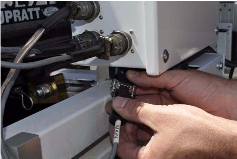
Figure 2-22. MC-R3 Main Antenna Serial Cable to RTP-300 Assembly
