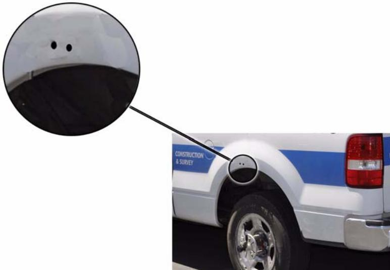
Figure 2-1. Wheel Encoder Bracket Location on Left Rear Fender
