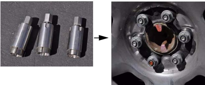
Figure 2-3. Lug Nut Mounts and Vehicle Lug Nuts - Before
