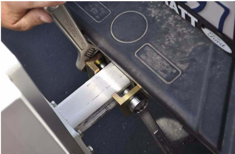
Figure 2-14. Install Hitch Mount Bracket Nut and Washer
