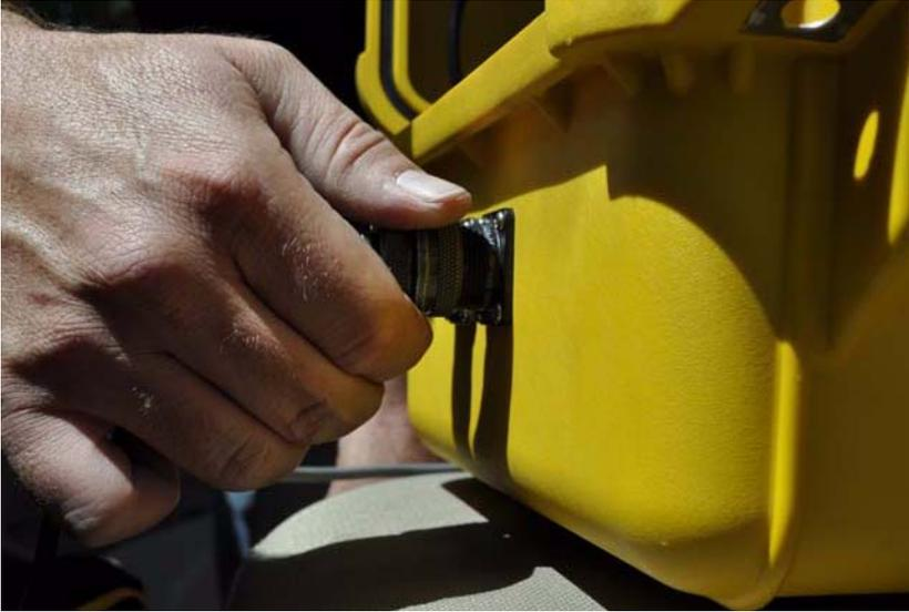
**Figure 2-28. RTP-300 Communication Cable to Pelican Case**
