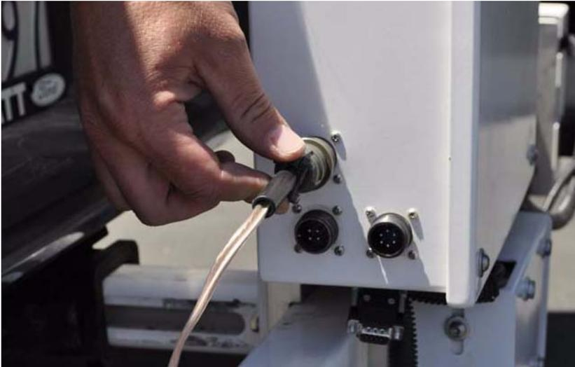
**Figure 2-18. Connect RTP-300 Power Cable to RTP-300 Assembly**
