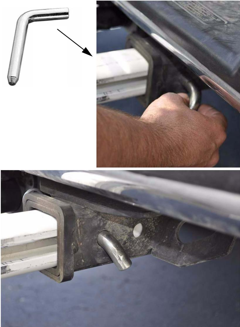
**Figure 2-10. Install Hitch Pin**
