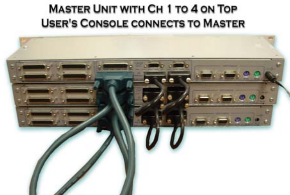
FIGURE 3 Stacking of MC4-H2 or MC4-H2-SW Units
