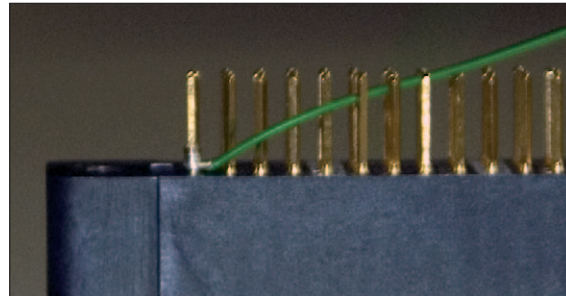
Figure B. Completed wrapped wire.
