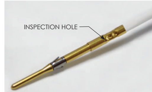
Figure E. The crimp region is between the inspection hole and the end.
