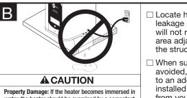
Property Damage: If the heater becomes immersed in water, the heater should be examined by a competent service person before it is placed back in operation. Locate heater in an area where leakage of the tank or connections will not result in damage to the area adjacent or to lower floors of the structure.
