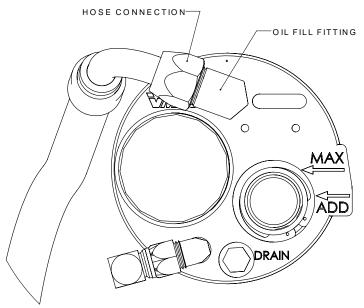
Figure 3 – Oil fill fitting location
