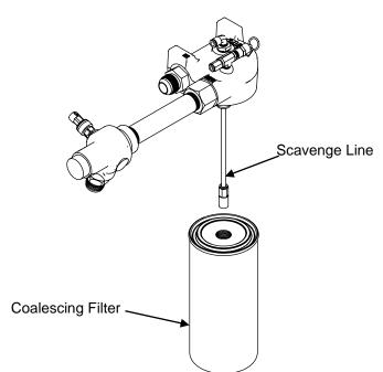
Figure 5 – Avoid Damaging the Scavenge Line
