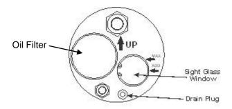
Figure 1 – Oil Drain, Filter and Sight Glass Location
