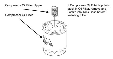
Figure 2 – Compressor Oil Filter
