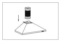
**Step 2**. Note. The unit is supplied with a wall bracket and a bracket that attaches to the Inner Duct. The wall bracket is secured to the wall and the hood then simply hooks onto the wall bracket when assembled.
