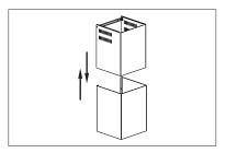
Step 4. Fit the duct cover to the hood body (M4 Screws)
