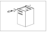
Step 3. Insert the inner duct cover into the outer duct cover
