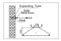
**Step 6**. Hang the complete range hood on the wall bracket. Ensure it is level.
