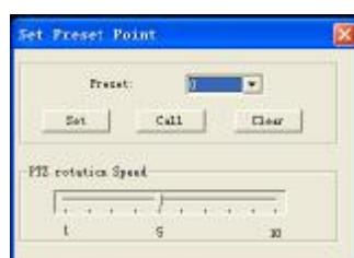
PTZ control: set up / call / clear preset points and set up pan&tilt head rotate speed, maximum 32 preset
