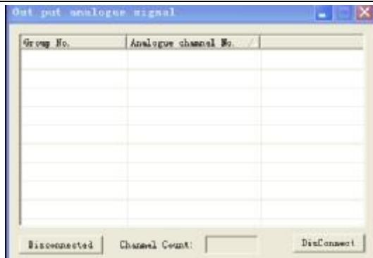
Select "connect video decode card" ( group number: current monitoring channel; analogue channel:output channel ), select analogue channel, the following dialog box pops up:
