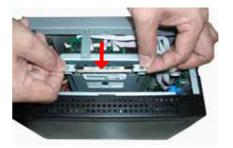
**Step 5** Fix the HDD bracket firmly into the HDD drive.
