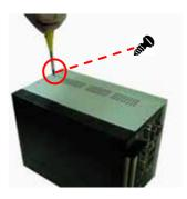
Step 4 Open the side cover and locate the Hard Disk Drive.
