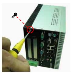
**Step 5** Align the PCI card with the slot, and latch the PCI bracket with the slot on the front panel.Press the card into the slot until it is firmly seated, and screw the PCI bracket onto the front panel.
