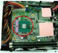
**Step 5** Place the heat sink on the CPU, and lock it down.
