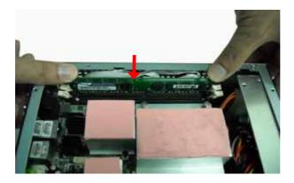
(2) Install the memory module into the socket and push it firmly down until it is fully seated. The socket latches are levered upwards and clipped on to the edges of the SO-DIMM.
