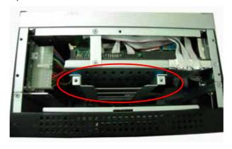
**Step 5** Use assembly parts to fix HDD with the bracket, and install the HDD.
