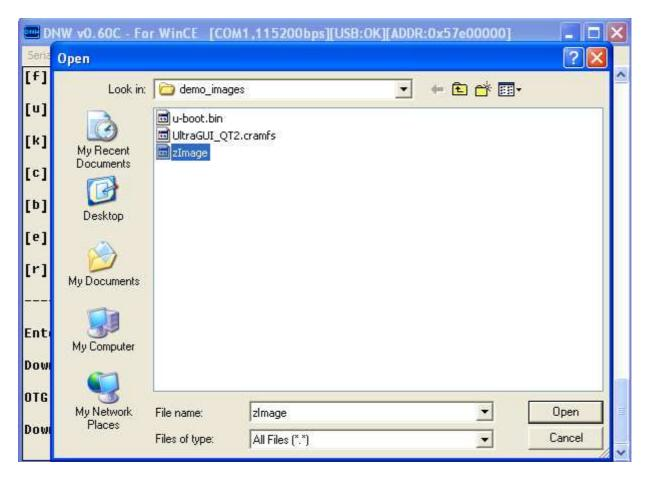
The Linux kernel will be downloaded and automatically burned to the NAND Flash.
