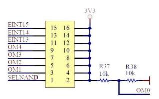
The signal SELNAND determines the type of NAND memory. It should be "1" (high power level) when using NAND Flash while "0" (low) when using ONENAND. On the *uConrol* Platform, we use NAND Flash; therefore the power level of the SELNAND signal is high.
