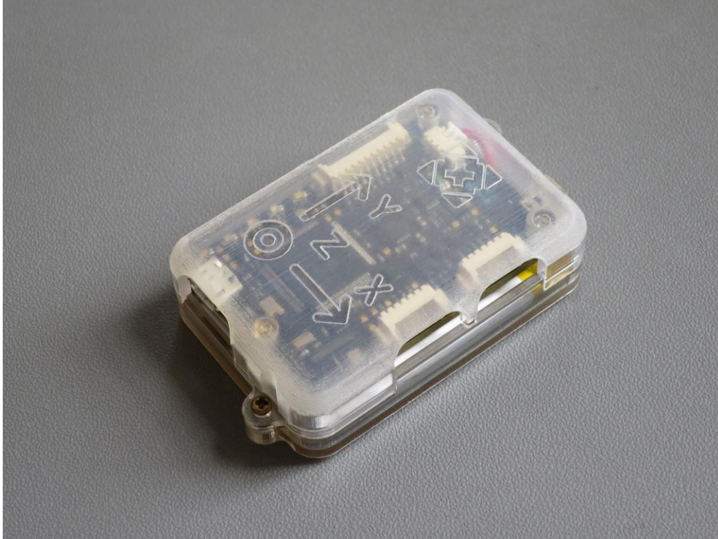
Figure 3: 3D printed prototype of the plastic housing
