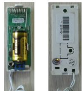
connect wireless emitter with metallic sensor via wired
