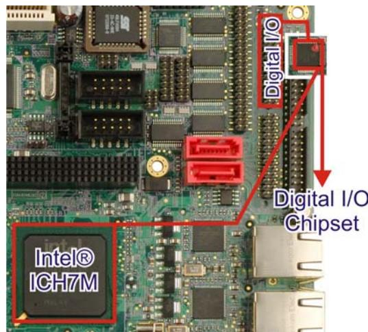
Figure 2-30: Lattice Semiconductor LC4064V Digital I/O Chipset
