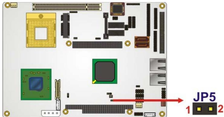
Figure 5-14: PC/104 Voltage Setup Jumper Pinout Locations
