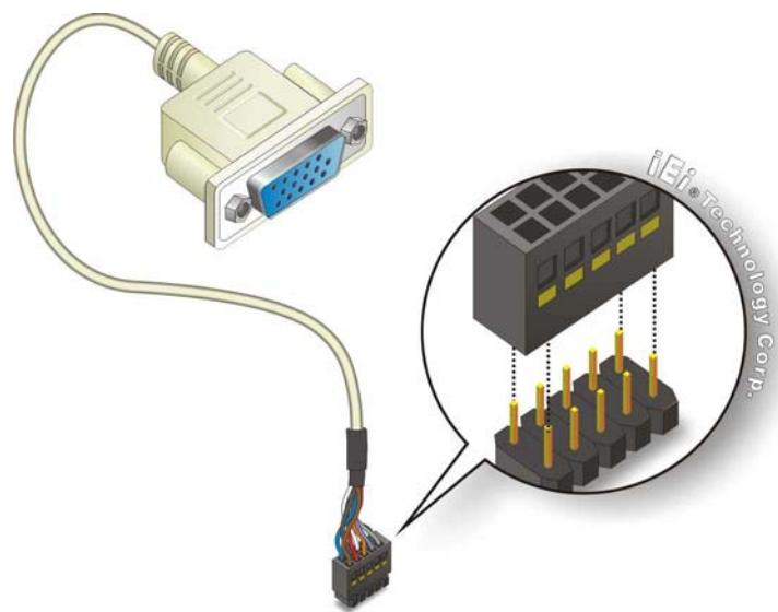
Figure 5-29: VGA Pin Header
