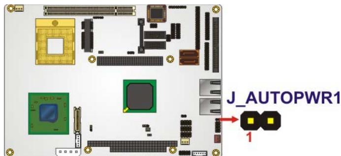
**Figure 5-9: Auto Power-on Function Setup Jumper Location**
