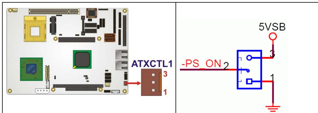
Figure 4-4: ATX Power Supply Enable Connector Location
