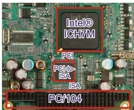
Figure 2-20: PC/104 Expansion Slot
