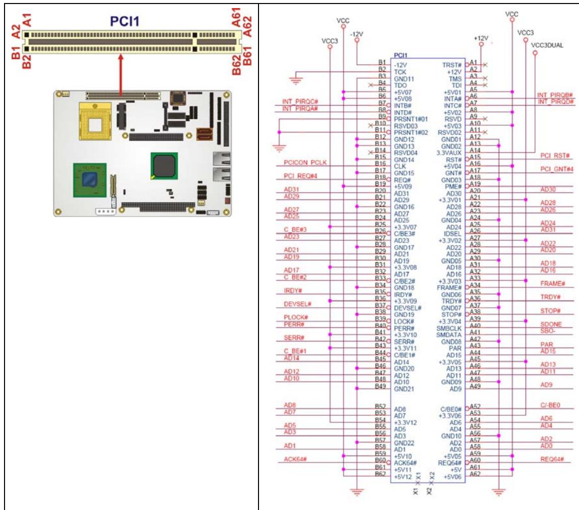
Figure 4-17: PCI Slot Location
