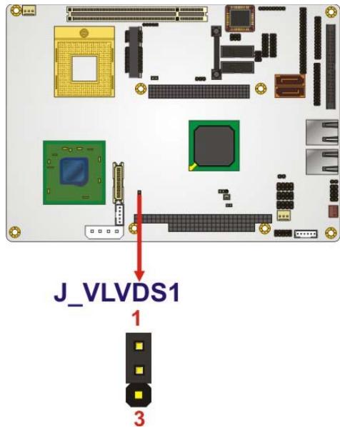
**Figure 5-12: LVDS Voltage Selection Jumper Pinout Locations**
