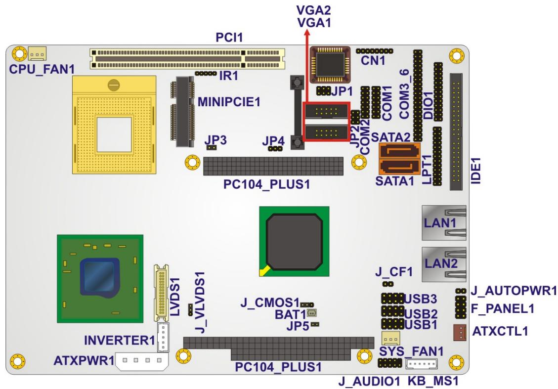
Figure 4-1: Connector and Jumper Locations
