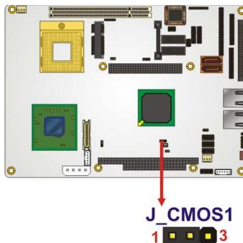
Figure 5-11: Clear CMOS Jumper
