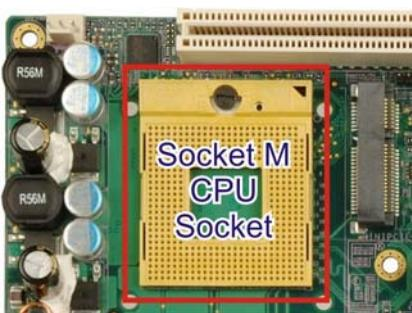
**Figure 2-4: Socket M CPU Socket**
