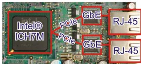
**Figure 2-22: Broadcom PCI GbE Controllers**
