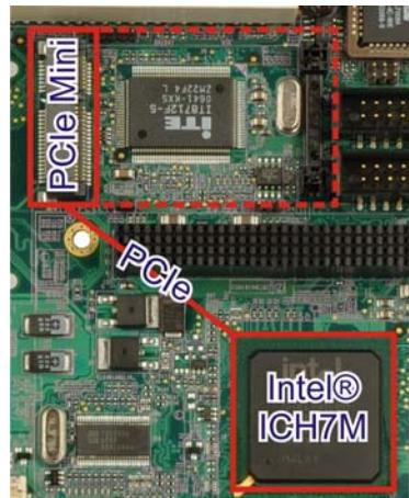
Figure 2-21: PCIe Mini Card Socket
