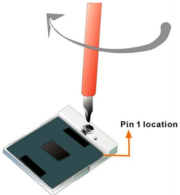
Figure 5-2: Lock the CPU Socket Retention Screw
