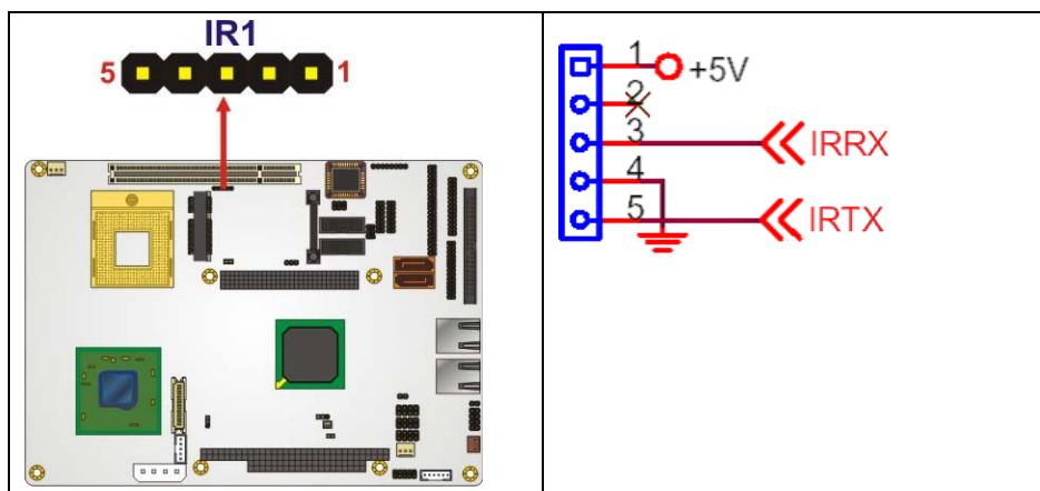
**Figure 4-11: Infrared Connector Pinout Locations**
