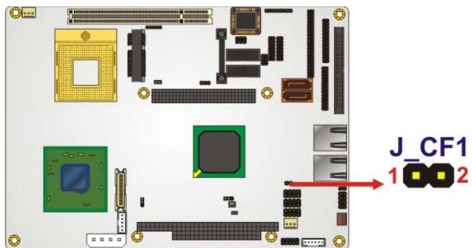
Figure 5-10: CF Card Setup Jumper Location
