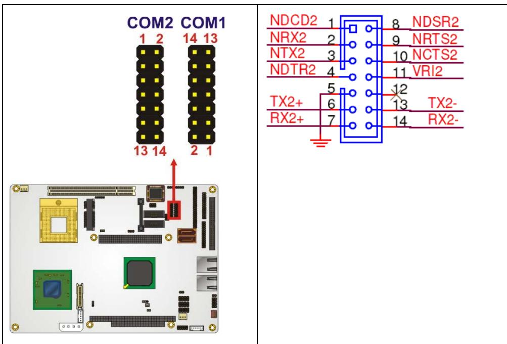
Figure 4-19: RS-232/422/485 Serial Port Connector Location
