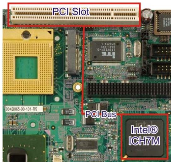
Figure 2-18: PCI Expansion Slot
