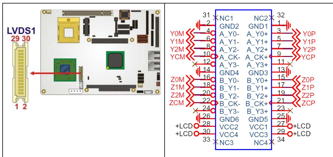
**Figure 4-14: LVDS LCD Connector Pinout Locations**
