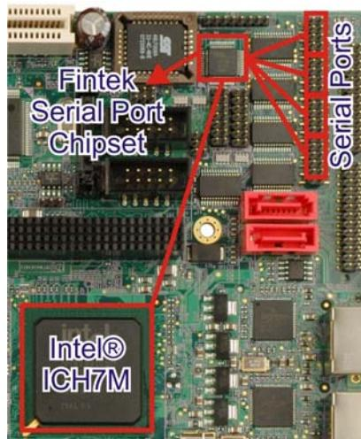
Figure 2-29: Fintek F81216DG LPC Serial Port Chipset
