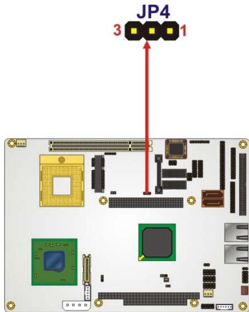
**Figure 5-16: PCI-104 Voltage Setup Jumper Pinout Locations**
