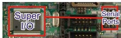
Figure 2-25: Serial Ports
