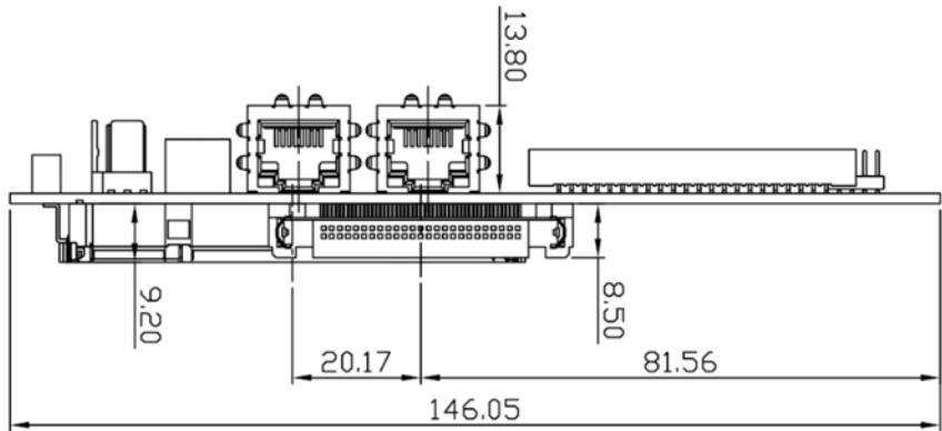
**Figure 2-2: External Interface Panel Dimensions (mm)**
