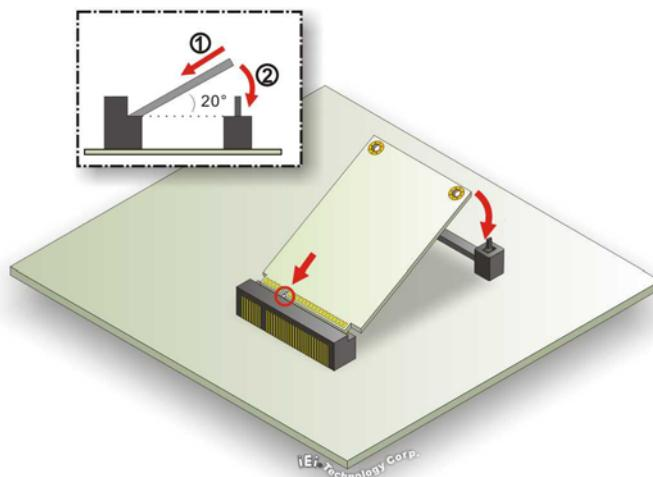
Figure 5-25: PCIe Mini Card Installation
