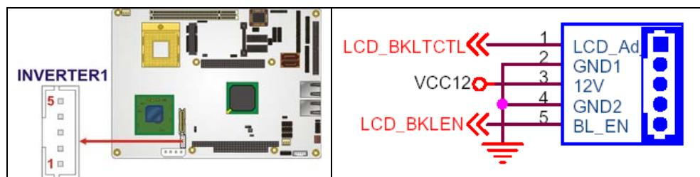
**Figure 4-12: Panel Backlight Connector Pinout Locations**
