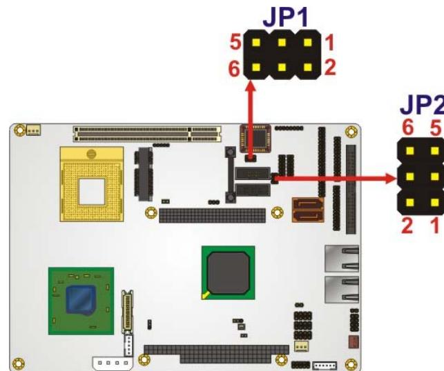
**Figure 5-15: Serial Port Mode Selector Pinout Location**
