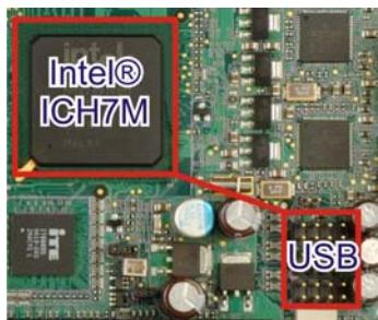
Figure 2-17: Onboard USB Implementation
