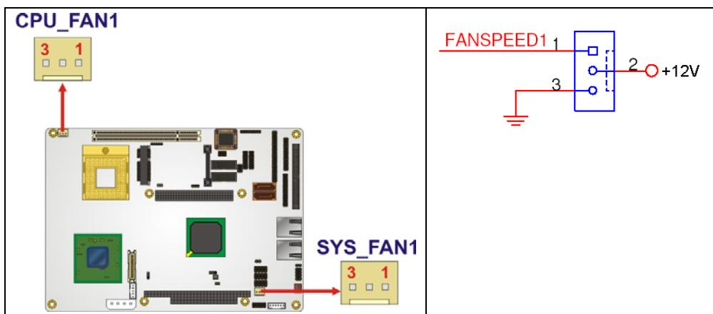
Figure 4-8: +12V Fan Connector Location
