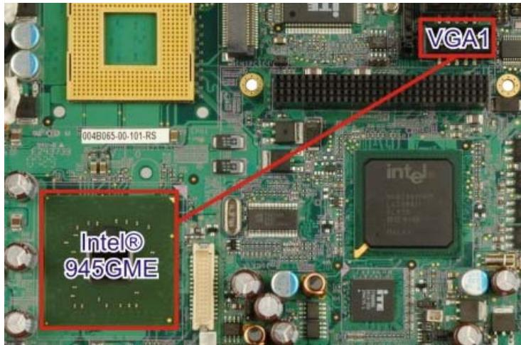
Figure 2-8: VGA Output
