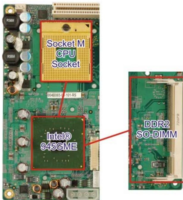
**Figure 2-6: 200-pin DDR2 SO-DIMM Socket**
