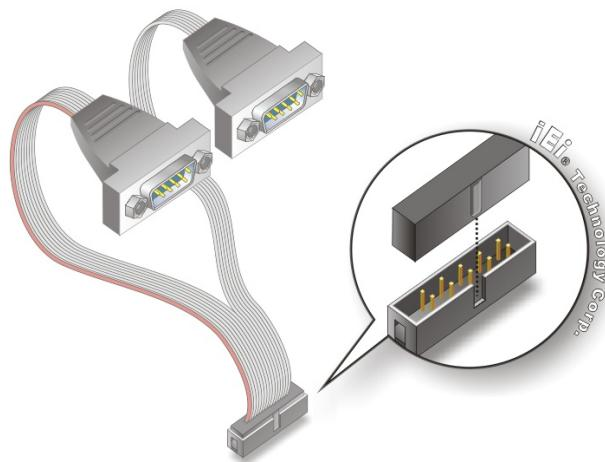
**Figure 5-27: RS-232/422/485 Cable Installation**
