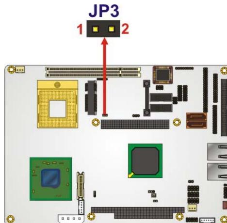
**Figure 5-13: PCI-104 Voltage Setup Jumper Pinout Locations**
