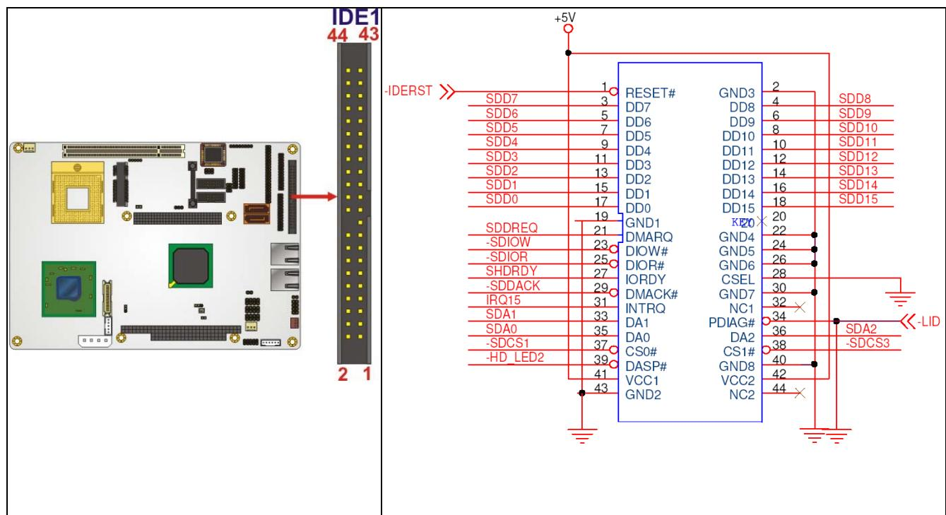
**Figure 4-10: Secondary IDE Device Connector Locations**
