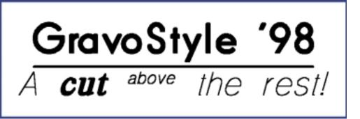
This job uses a 0.030" Gravoply tool for the bold letters and a 0.010" Gravoply tool for the thin letters. WYSIWYRE is a tool to help you can see if your chosen tool(s) yields the desired effect.
