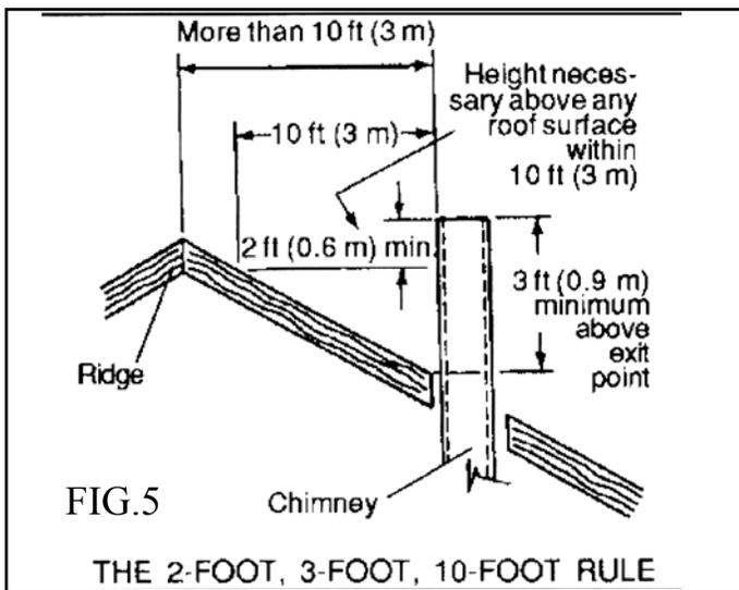
Limit connector pipe to 8 ft. or less, with no more than two elbows. All horizontal sections should have 1/4 in. rise per foot. The chimney must be capable of providing a draft reading of at least .06 in. of water column. A barometric damper can be installed to prevent excessive and erratic draft. All connector pipe should be secured with sheet metal screws at each joint.
