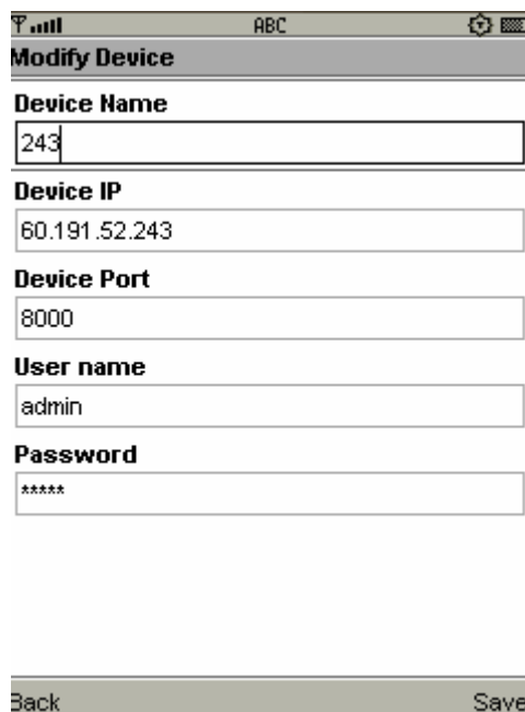
Fig. 2-6 Interface for modifying the device
