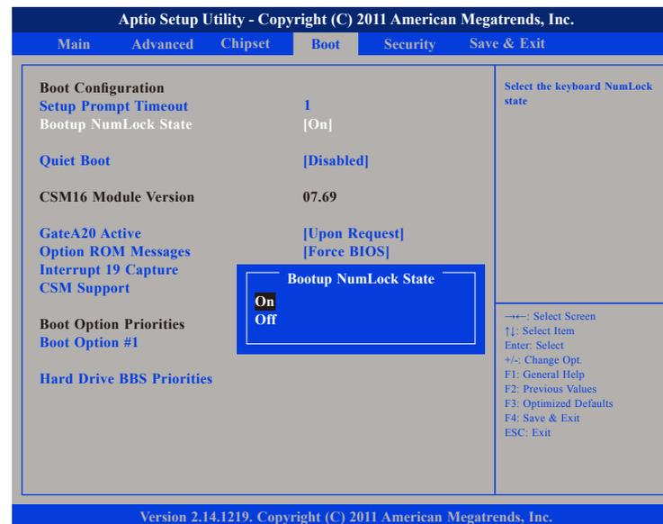
This allows you to determine the default state of the numeric keypad. By default, the system boots up with NumLock on wherein the function of the numeric keypad is the number keys. When set to Off, the function of the numeric keypad is the arrow keys.
