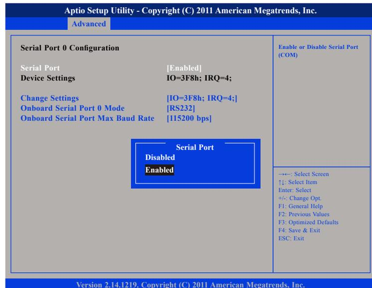
This field is used to enable or disable the serial port.
