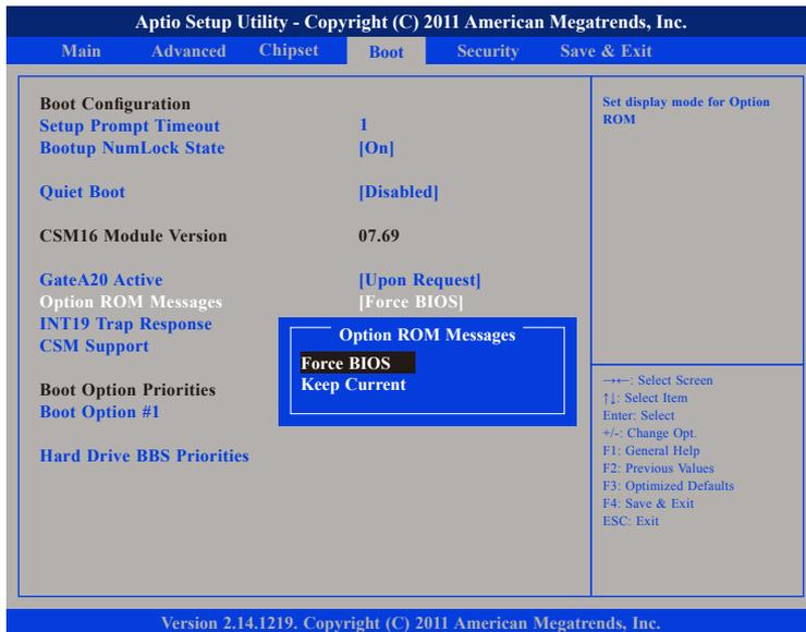
This field is used to set display mode for Option ROM. The options are Force BIOS and Keep Current.
