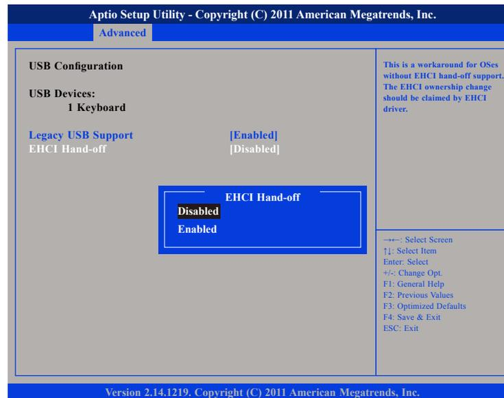
This is a workaround for OSes that does not support EHCI hand-off. The EHCI ownership change should be claimed by the EHCI driver.
