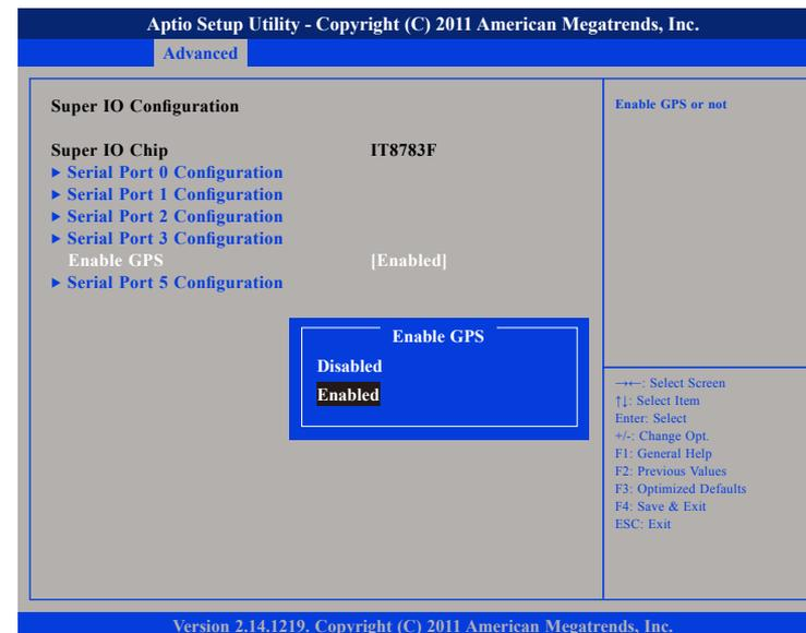
This field is used to enable or disable GPS.
