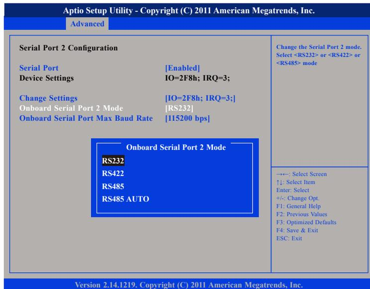
This field is used to configure the mode of serial port 2 as RS232, RS422, RS485 or RS485 AUTO.
