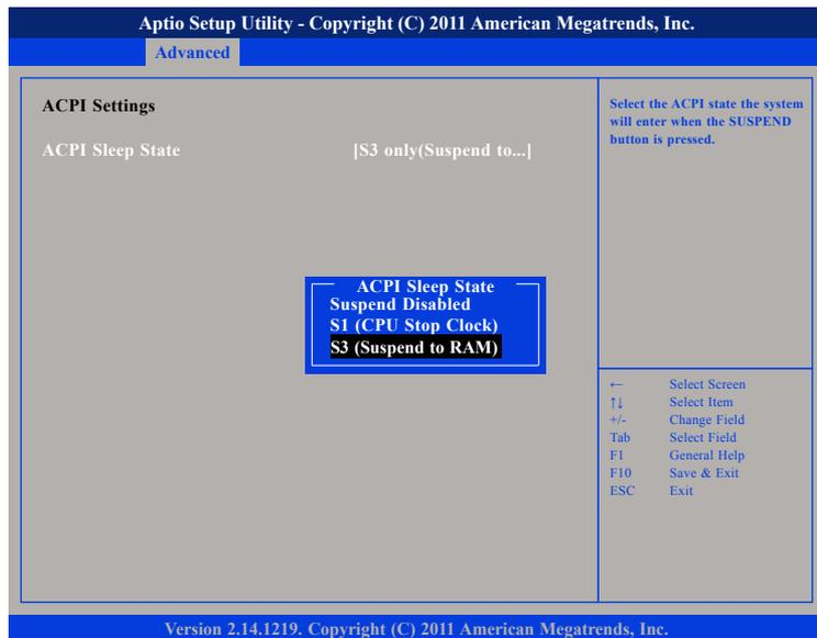
Select the highest ACPI sleep state the system will enter when the suspend button is pressed. The options are Suspend Disabled, S1 (CPU Stop Clock) and S3 (Suspend to RAM).
