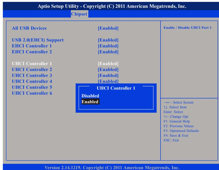
These fields are used to enable or disable UHCI port 1 to port 6.
