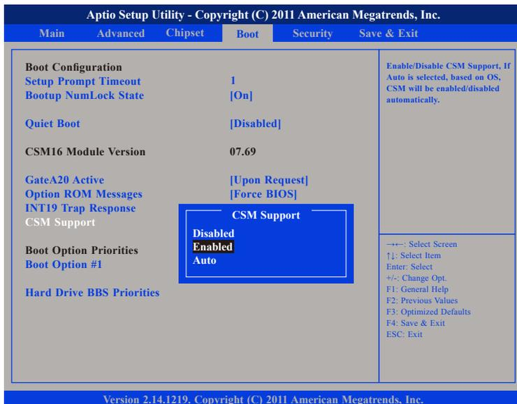
This field is used to enable or disable CSM support, if Auto option is selected, based on OS, CSM will be enabled or disabled automatically.
