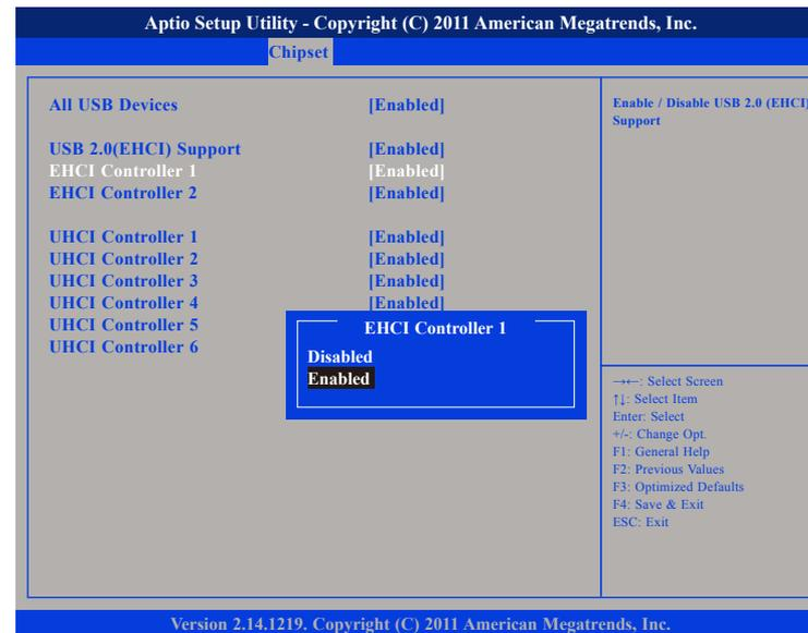
These fields are used to enable or disable USB 2.0 (EHCI) support for controller 1 and 2.
