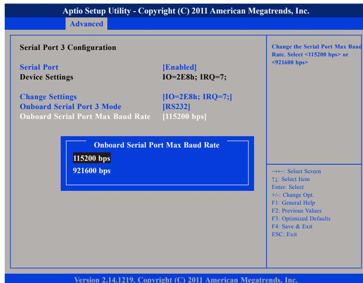
This field configures the maximum baud rate of the serial port 3, the options are 115200 bps and 921600 bps.
