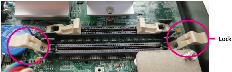
3. Insert the module into the socket at an 90 degree angle. Apply firm and even pressure to each end of the module until it slips into the socket.
