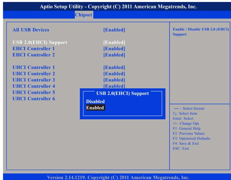
This field is used to enable or disable USB 2.0 (EHCI) support.
