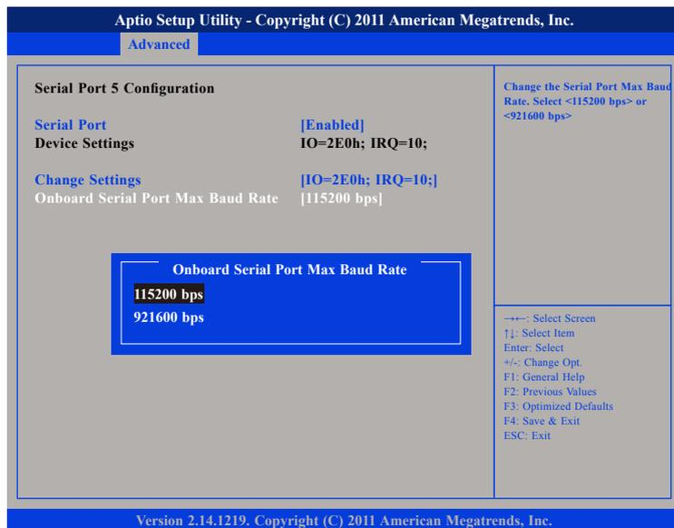
This field configures the maximum baud rate of the serial port 5, the options are 115200 bps and 921600 bps.
