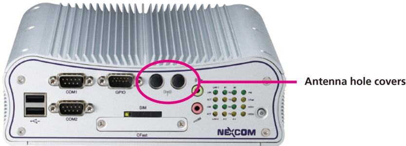
2. Insert the antenna jack end of the cable through the antenna hole.
