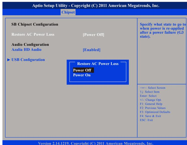
**Power Off** When power returns after an AC power failure, the system's power is off. You must press the Power button to power-on the system.
