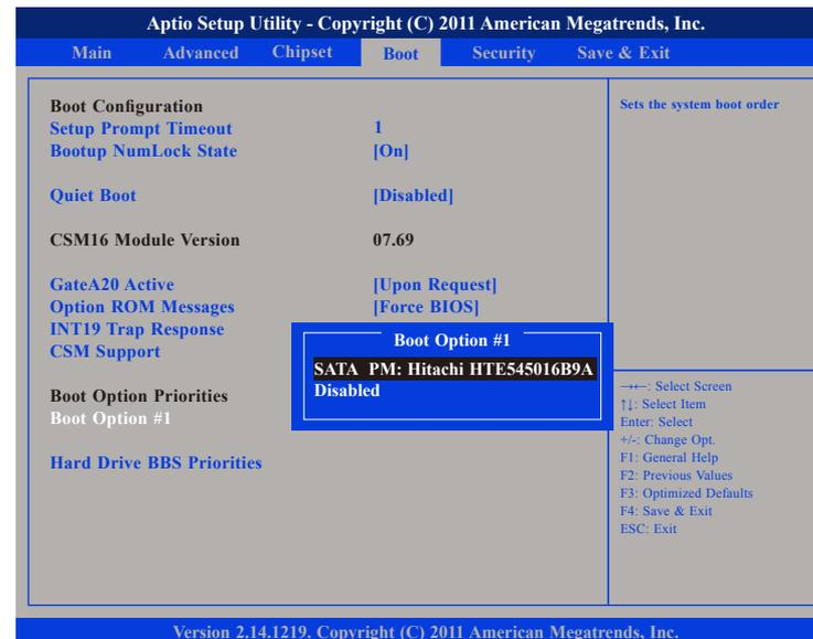
This field is used to adjust the boot sequence of the system. Boot Option #1 is the first boot device that the system will boot from, next will be #2 and so forth.
