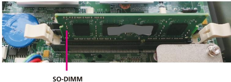
4. While pushing the SO-DIMM into the position, the lock will close automatically.
