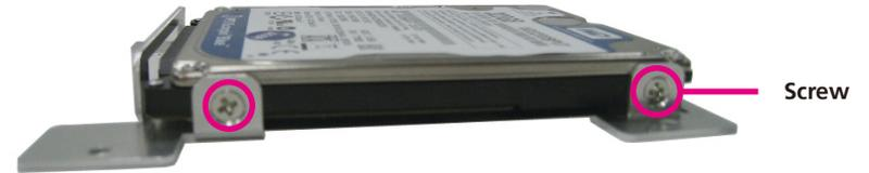
3. Connect the SATA data/power cable and secure the cable with provided screws.
