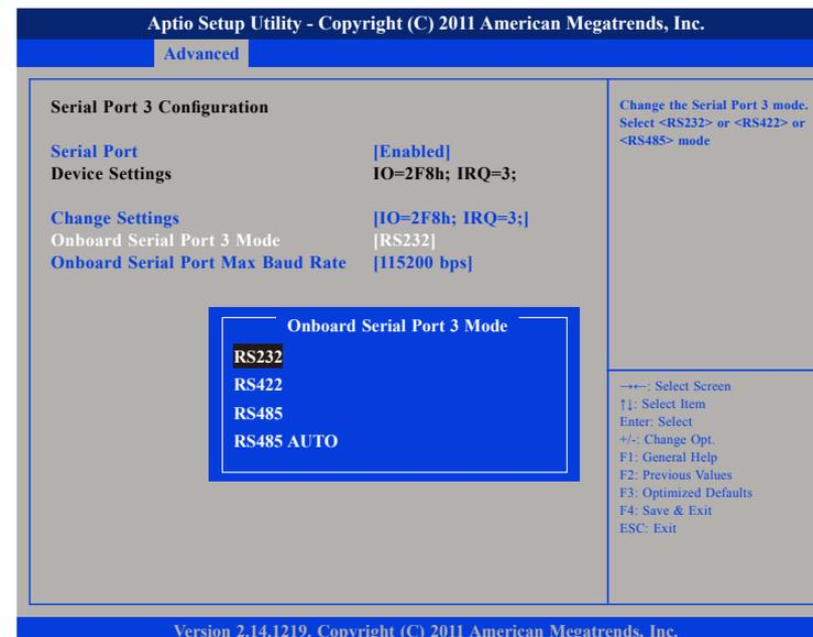
This field is used to configure the mode of serial port 3 as RS232, RS422, RS485 or RS485 AUTO.
