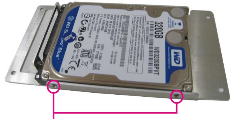
Screw to fasten HDD drive
