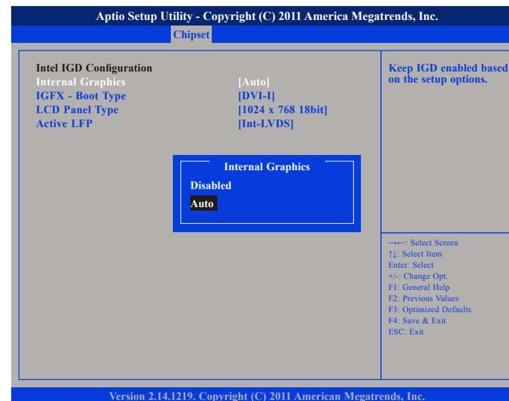
This field is used to disable or enable the internal graphics.
