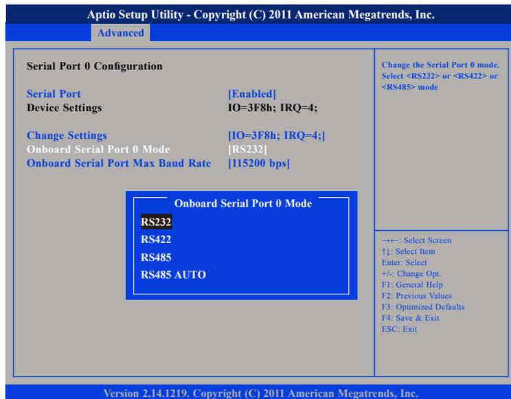
This field is used to configure the mode of serial port 0 as RS232, RS422, RS485 or RS485 AUTO.
