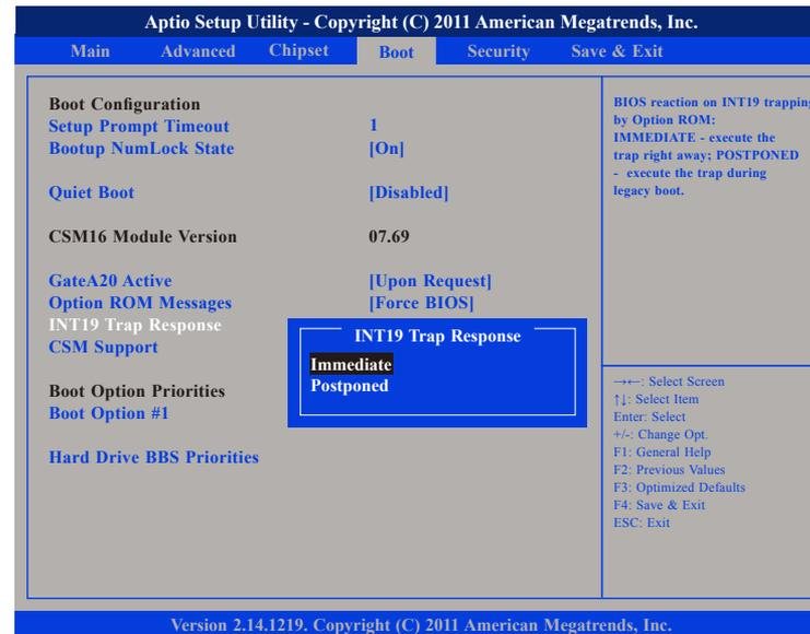
Allows Option ROMs to trap Interrupt 19 when enabled.
