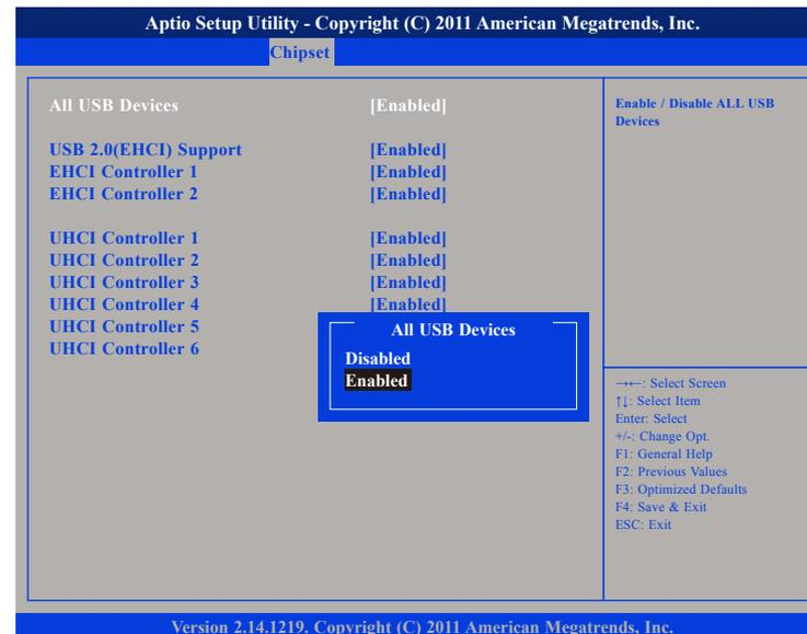
This field is used to enable or disable all the USB devices.
