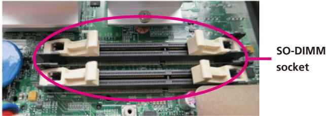
2. Release the lock of the SO-DIMM socket.
