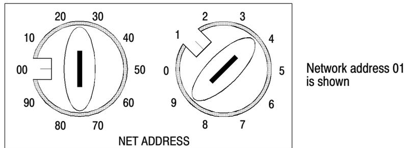
**Tip** For optimum throughput, assign addresses to your ControlNet nodes in a sequential order starting with 01 for the controlling processor.
