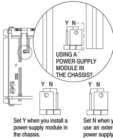
1. Locate the chassis configuration plug (between the two left most slots of the chassis).
