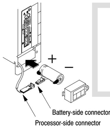
To **install** the battery, slide the battery-side connector into the processor-side connector until you hear them snap.
