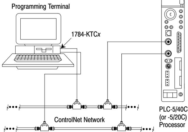
**Using 1784-KTC or -KTCx communication card and NAP<sup>①</sup>**
