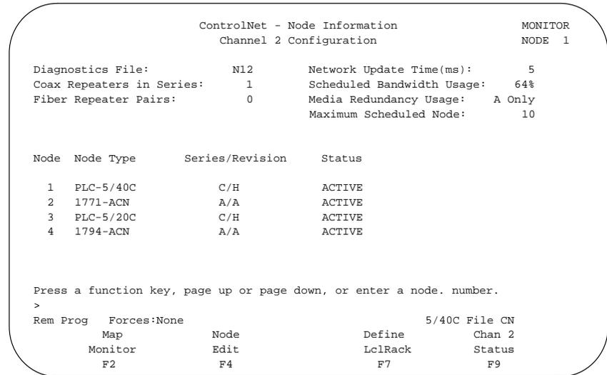
The ControlNet Node Information (Monitor) screen lists the nodes that you have entered for the ControlNet network; and it shows the node type, product series/revision, and status (active or inactive) that you have configured for each node.
