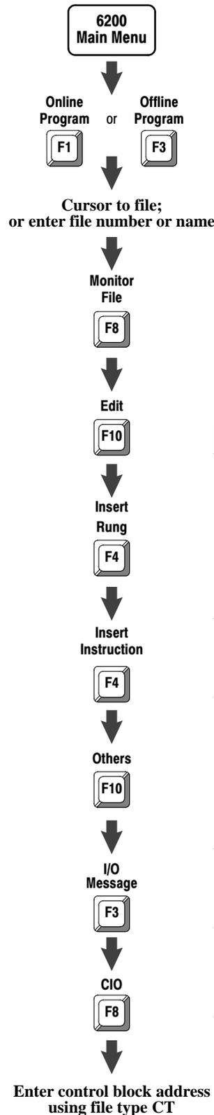
You can use the ControlNet I/O Transfer (CIO) instruction and the ControlNet Transfer (CT) data type to make ControlNet I/O transfers within the local ControlNet link. Follow the steps on the left to go to the Instruction Entry for ControlNet I/O Transfer Block screen.
