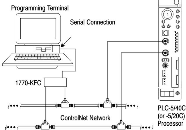
**Using 1770-KFC communication interface and NAP<sup>①</sup>**
