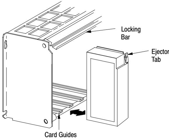
**ATTENTION:** Make certain that power to the chassis is off before inserting or removing the processor.
