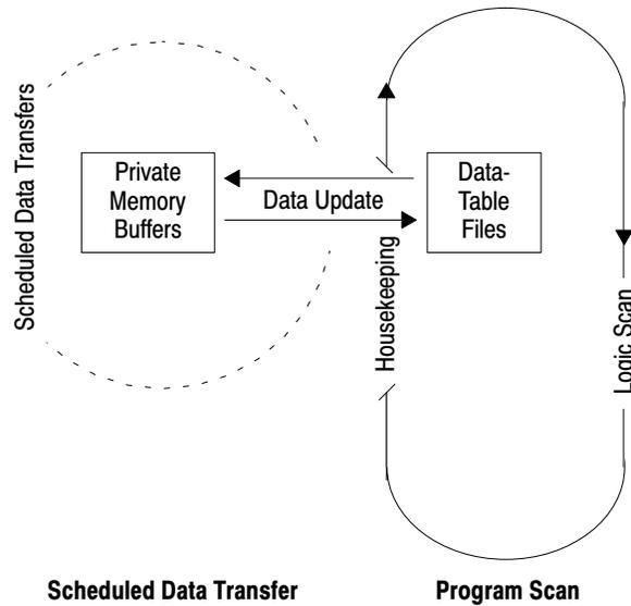
The following scheduled data-transfer operations are supported by the PLC-5/20C and -5/40C processors on a ControlNet network:
