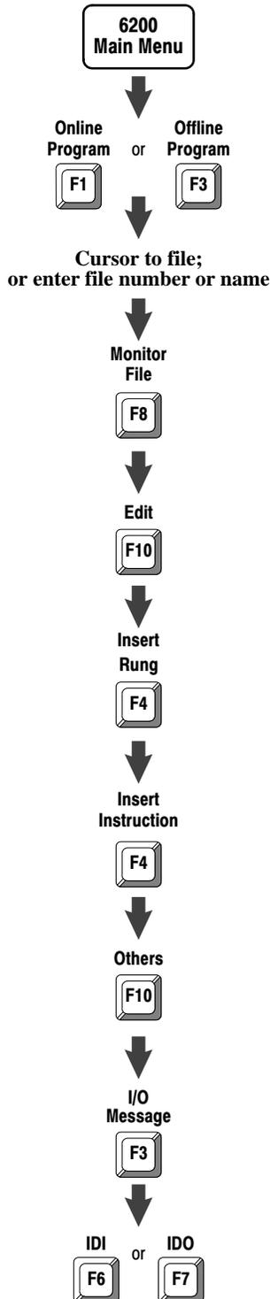
You can use two instructions for immediate data input and output on a ControlNet network—Immediate Data Input (IDI) and Immediate Data Output (IDO).
