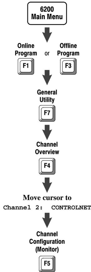
Follow the steps on the left to go to the ControlNet Node Information (Monitor) screen. If the ControlNet information in the processor does not match that on the current ControlNet link, the software redisplay the Channel Overview screen with a new prompt and set of function keys.
