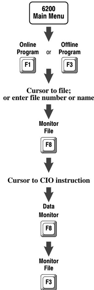
Follow the steps on the left to go to the Data Monitor for ControlNet I/O Transfer Block screen.
