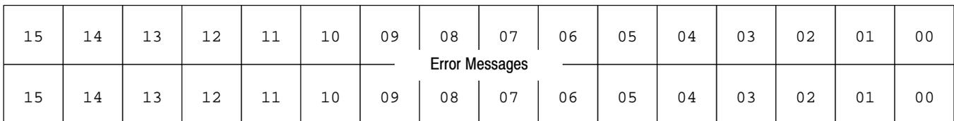
If these status words are for a 1794 Flex I/O module and there is no connection error, any 1's set in bits 00 through 07 of the third word indicate errors in the corresponding slots (numbered 0 through 7)
