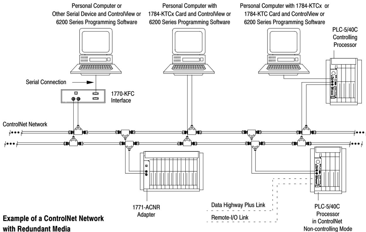
**Example of a ControlNet Network with Redundant Media**
