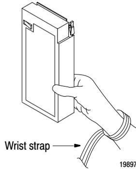
Your processor is shipped in a static-shielded container to guard against electrostatic damage. Electrostatic discharge can damage integrated circuits or semiconductors in the processor if you touch backplane connector pins. It can also damage the module when you set configuration plugs or switches inside the module. Avoid electrostatic damage by observing the following precautions.
