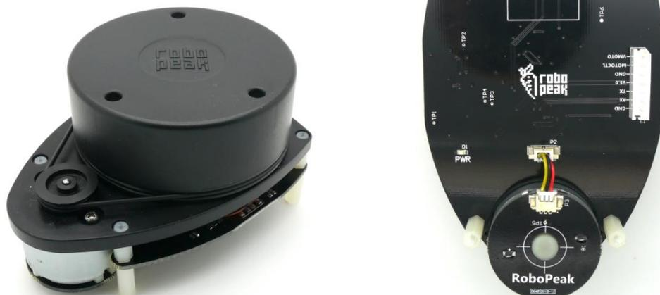
RPLIDAR development kit contains standard RPLIDAR unit (A1M1-R1). The RPLIDAR embedded logic IO drivable (3.3V) motor controller which can be used to configure scan frequency by tuning motor speed. Developer also can choose to turn off motor for power saving purpose.
