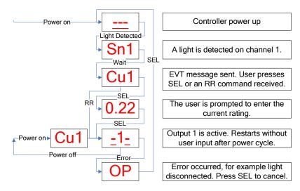
The main alternating display on the front panel will show a "1" when channel 1 has a light connected and "2" when channel 2 has a light connected.
