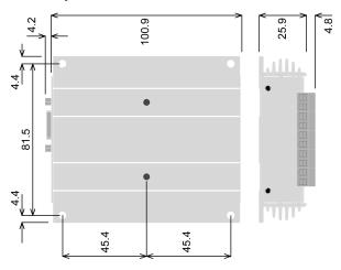
The PP500 can be mounted from above using the corner holes, or from beneath using the M4 tapped holes (maximum screw length inside is 6mm).
