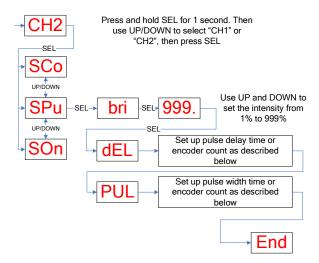
If a brightness greater than 100% is selected, the pulse width will be limited to a safe value as in the table in Section 4.3.2.
