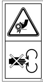
Do not open or remove safety guards while the feeder is connected to the tractor
