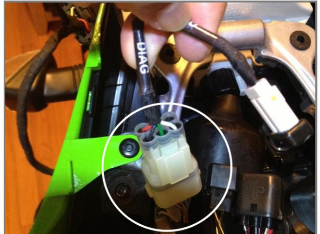
To connect SoloDL to your Kawasaki ZX10R Racing kit ECU use CAN OUTPUT connector placed under the bike windscreen.
