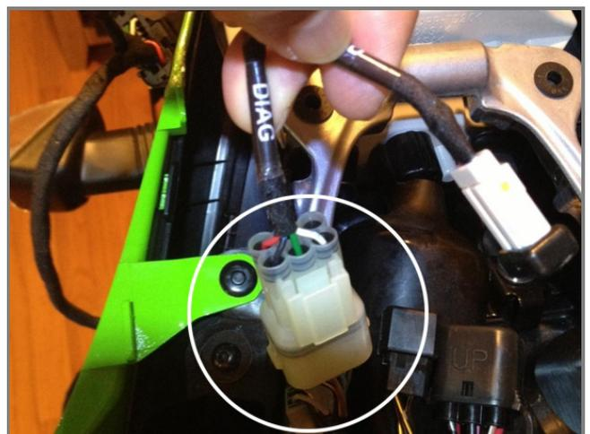
To connect EVO4 to your Kawasaki ZX10R Racing ECU kit use "CAN output" connector placed under the bike windscreen.
