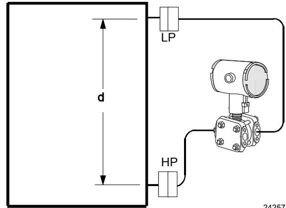
**Figure 18**—Density, direct acting transmitter configuration
