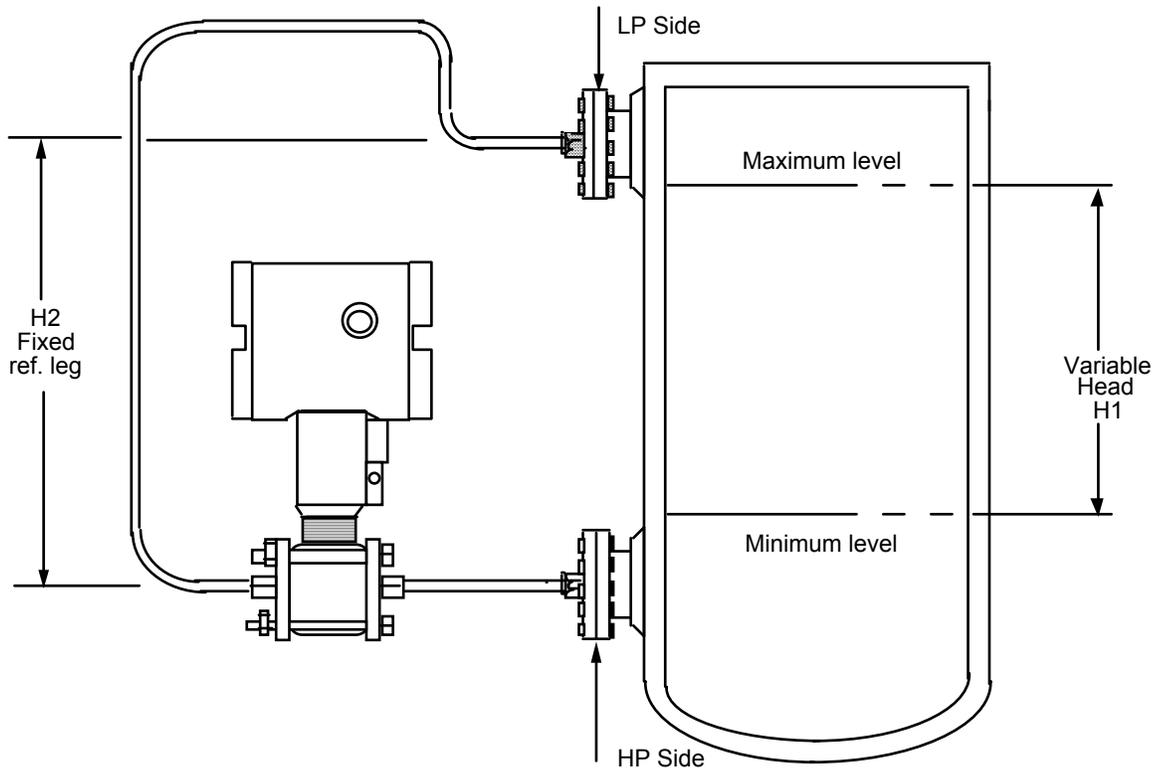
NOTE: Lower flange seal should not be mounted over 22 feet below the transmitter for silicone fill fluid (11 feet for CTFE fill fluid) with tank at one atmosphere. The combination of tank vacuum and high pressure capillary head effect should not exceed 9 psi vacuum (300 mmHg absolute).
