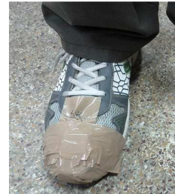
Figure 12: MIMU22BT on toes (preferred)
