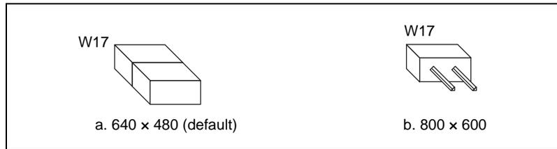
**Figure 3-6.** LCD Resolution Setting
