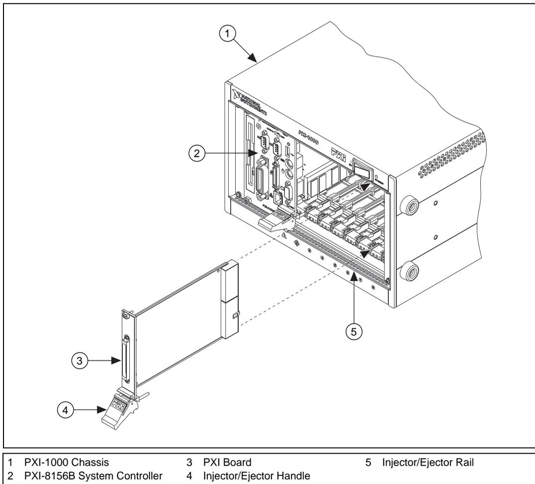
**Figure 3-12.** PXI-8156B Installed in a PXI Mainframe
