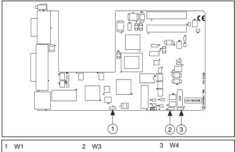
**Figure 3-1.** PXI-8150B Series I/O Board Parts Locator Diagram
