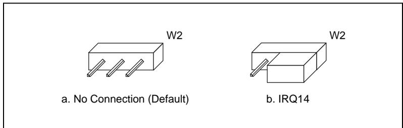
**Figure 3-9.** INTP Configuration
