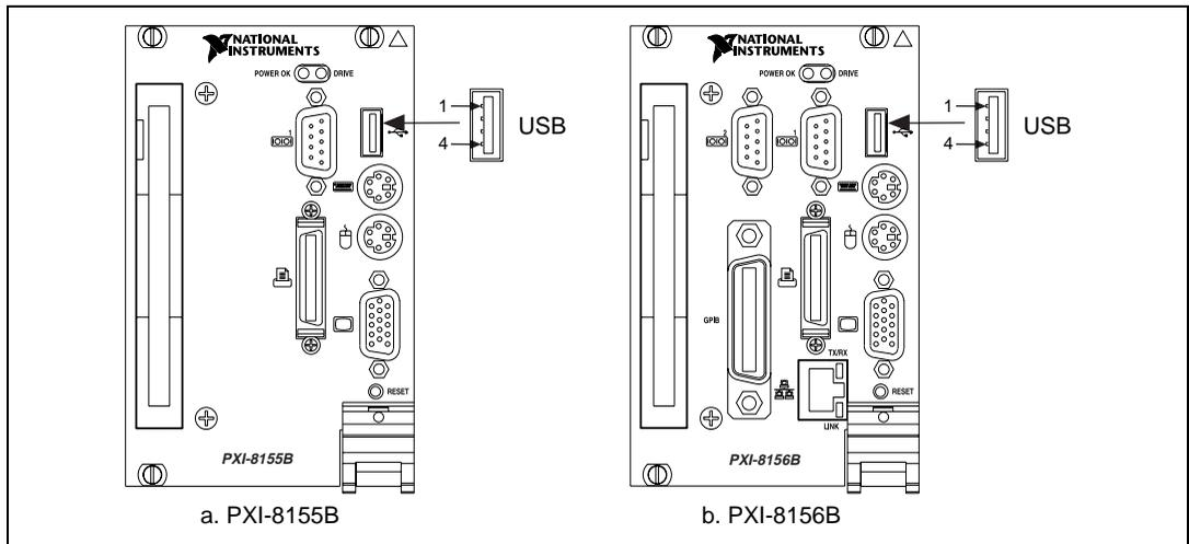
**Figure D-9.** USB Connector Location and Pinout**Table D-7.** USB Connector Signals
