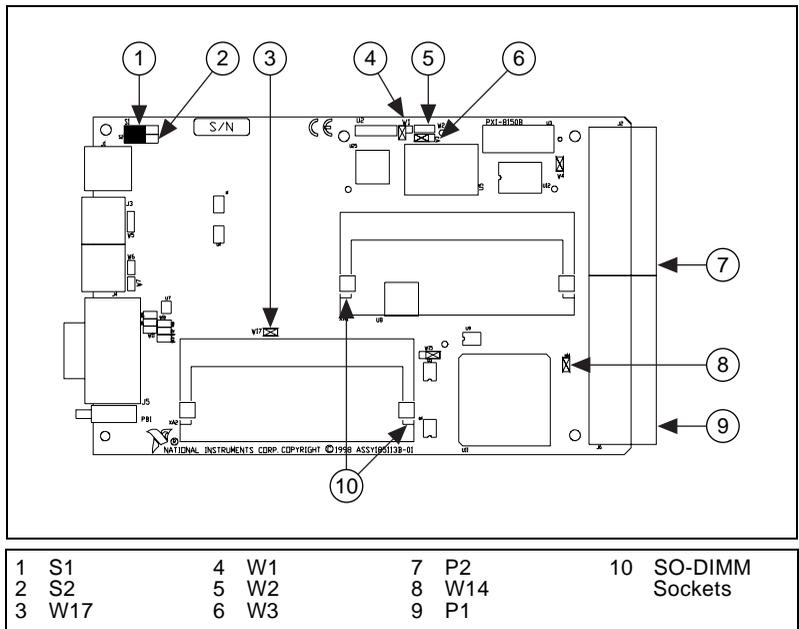
**Figure 3-2.** PXI-8150B Series CPU Board Parts Locator Diagram
