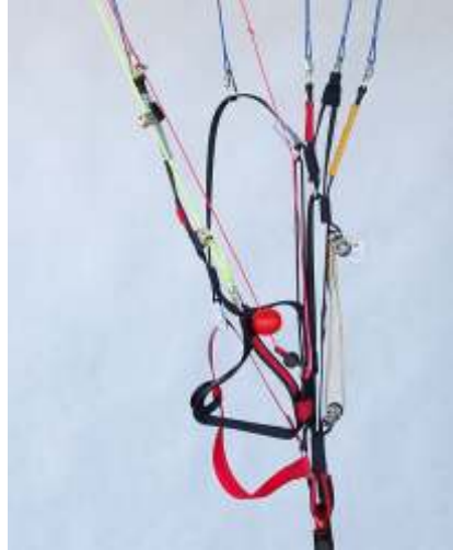
Figure 3 Additional magnet for brake handle (high hangpoints).
