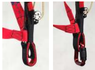
Figure 5 Beside TEA there is an additional inner loop in the risers that can be used for countering the torque effect. There is no adjustment possibility though, while in the TEA you can have the knot in just right place.
