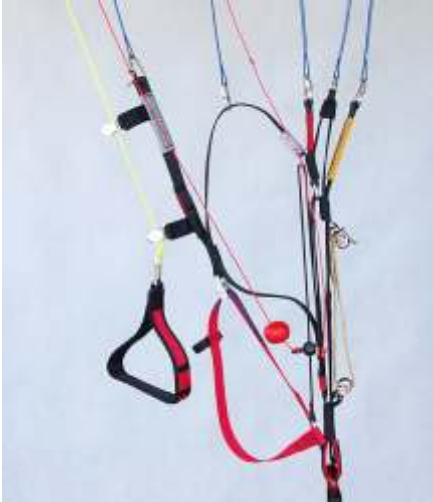
Figure 4 TEA cord inactive (a) and engaged (b)
