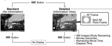
The AF frame changes according to its On/Off setting. (LCD monitor On)
